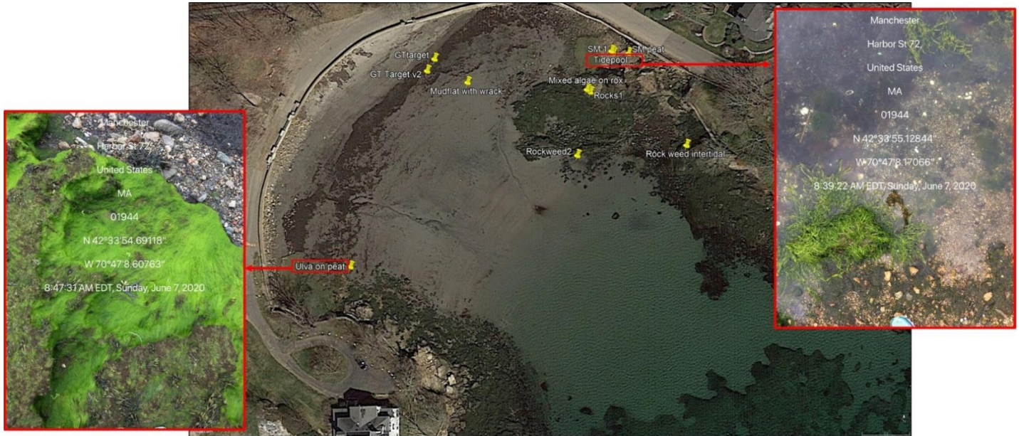
Figure 4. Example of groundtruthing data from Manchester Harbor (6/7/20). Data sources: cell phone photographs collected via My GPS Coordinates app, overlaid on Google Earth satellite imagery.
